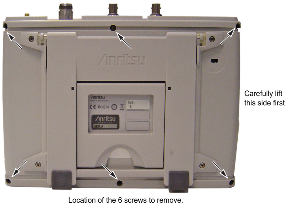
Figure 5-2. Remove the Six Screws
